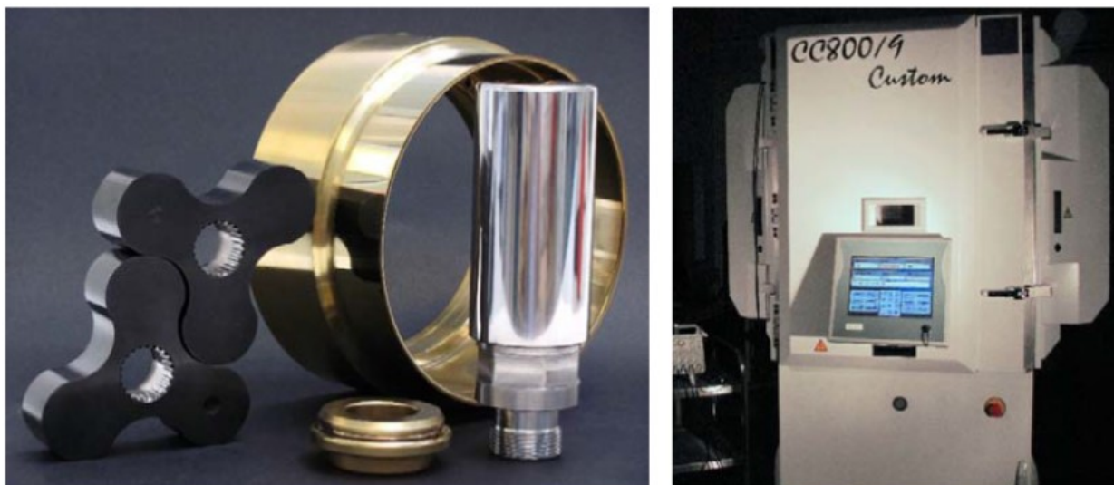
Figure 5 - To the left are seen different machine components PVD-coated with diamond-like carbon, TiN and CrN. To the right is seen a special customized HiPIMS (High Power Impulse Magnetron) PVD unit from CemeCon AG customized for the Danish Technological Institute. (Refer to Reference 1 for further details).
